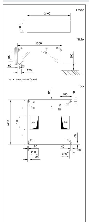
**Electric** Supply voltage: 641260 (STPF1524) 220 V/1N ph/50 Hz **Total Watts:** 0.16 kW Capacity: Supply capacity: 2400 m<sup>3</sup>/h **Key Information:** External dimensions, Width: 2400 mm External dimensions, Depth: 1500 mm External dimensions, Height: 500 mm Net weight: 160 kg Air Emission:
